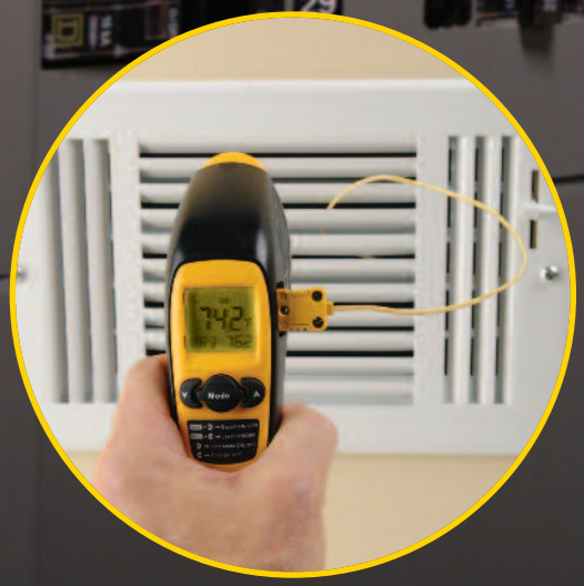
K-type thermocouple probe measures temperatures in hard-to-reach locations
